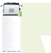
The cornering assistant is active at a speed of 0 to 30 km/h.
